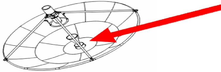
*Figure. 3 : Secondary Reflector*
