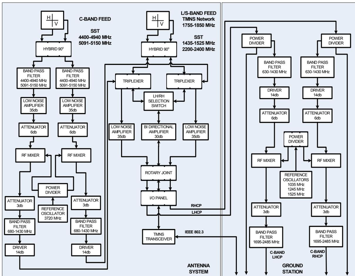
Figure 2: iNET Multi-Band Receiving Antenna Concept
